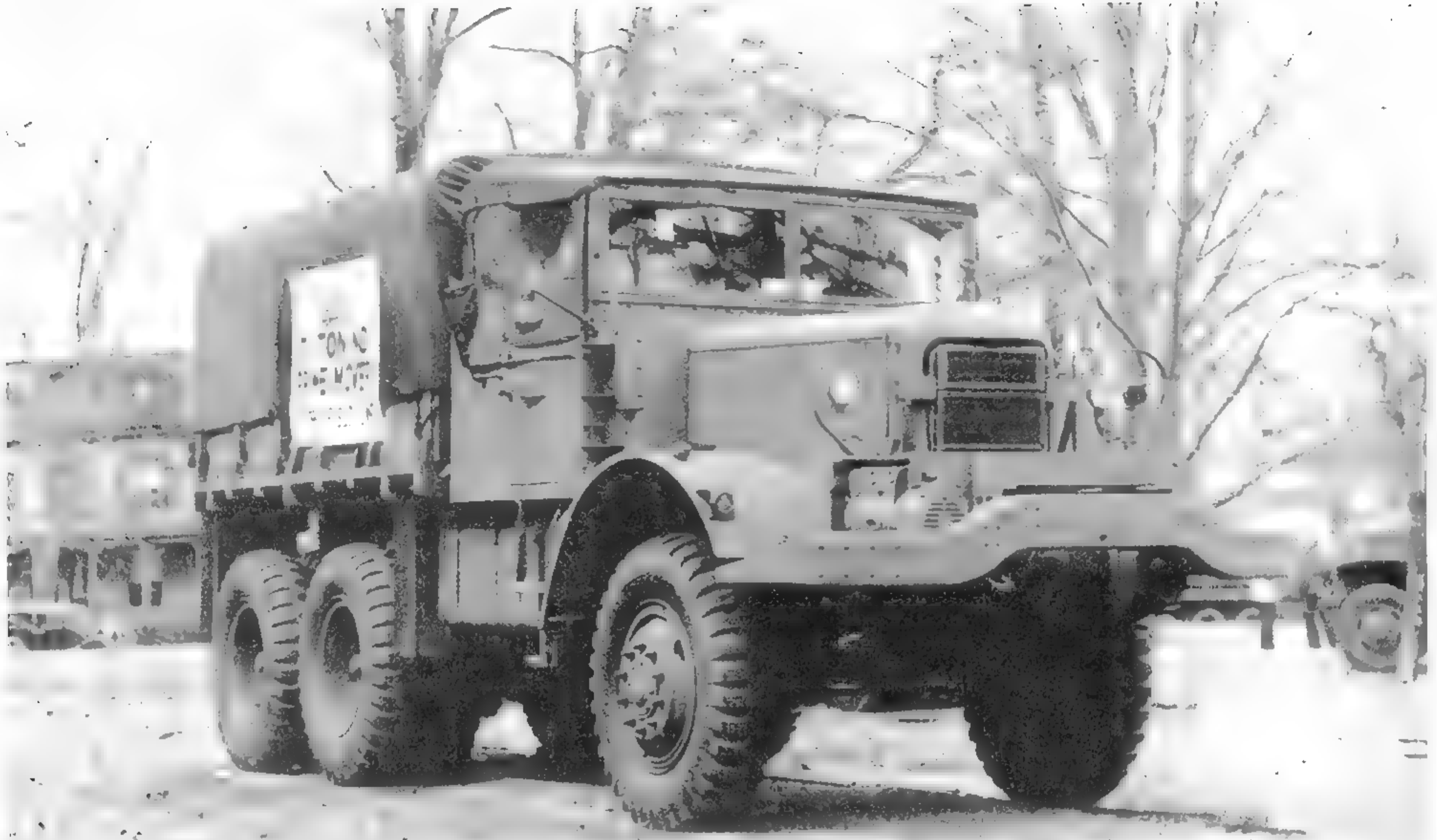
Although the NO-3s were all supplied for foreign aid, before shipping out this one took part in a War Bonds Drive. Notice the boards protecting the ground from the NO's weight (almost 30,000 lbs.), and the wide five-man cab. (Photo courtesy Mack Trucks Historical Museum)
